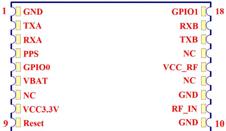
Figure 2: GT-1110-MT Pin Package
